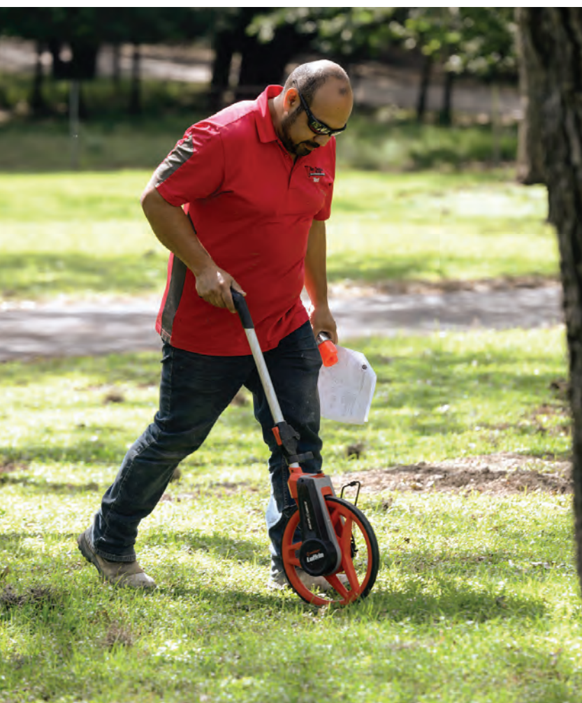
✓ Ted Talavara uses a Lufkin measuring wheel to mark trench lines during an installation.
